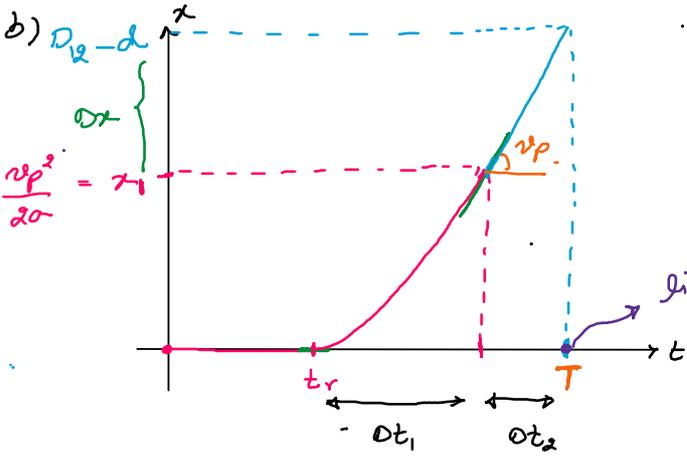
acceleration phase:  $v - v_0 = at \Rightarrow dt_1 = \frac{v_p}{a}$
