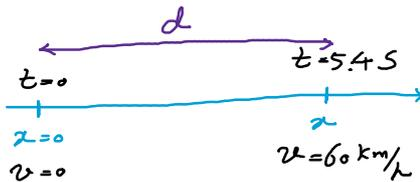
$$x = \frac{1}{2} a t^2 + v_0 t + x_0 \Rightarrow x = \frac{1}{2} \times 3.086 \times (5.4)^2 \approx 44.99 \approx 45 \text{ m}$$
