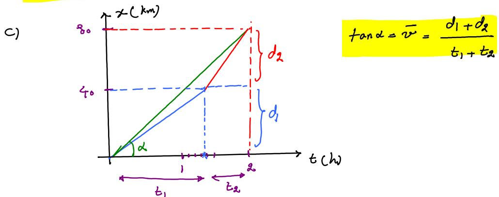
4 E A car moves uphill at 40 km/h and then back downhill at 60 km/h. What is the average speed for the round trip?
